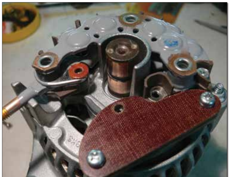
(Left) The mounting block is 1/4-inch thick and replaces the regulator after being cut to shape. It's made from two 1/8-inch thick pieces of canvas Bakelite, epoxied together and holding the nut. (Right) The mounting block attached to the alternator. Put one fiber washer where the left-hand brush-holder terminal was attached.
