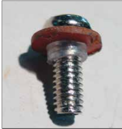
Assemble one fiber washer and the nylon tube on an M4x10-mm screw (left), then add a new wire terminal with a 5-mm hole, and fit the screw into the now 5-mm hole in the brush holder.
