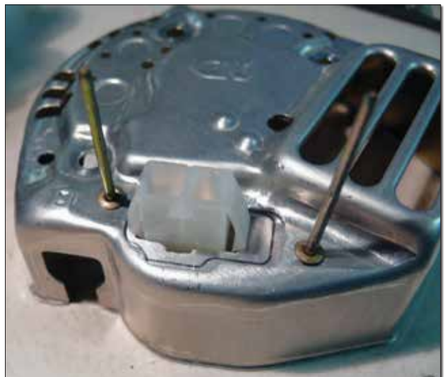
An alternative to having wires coming out of the cover is to mount a Molex-style terminal to the cover and attach it with two pop-rivets.
