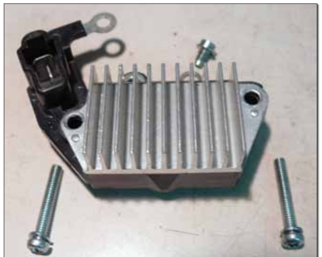
(Left) The brush holder is held in place with two screws. (Right) The alternator after removing the brush holder.
