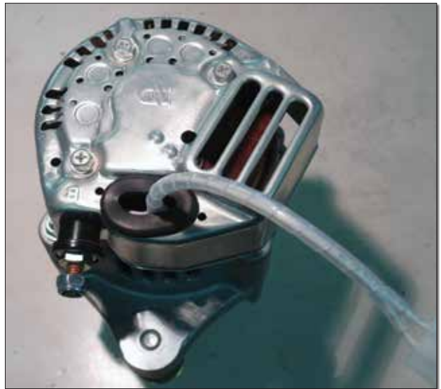
(Left) The brush holder mounted on the alternator with the right-hand new wire under the brush-holder lug. This keeps the brush holder precisely level and only a tiny fraction higher than the original position. (Right) Alternator with terminal shroud reinstalled and wires threaded through a rubber grommet fitted to the rear cover.
