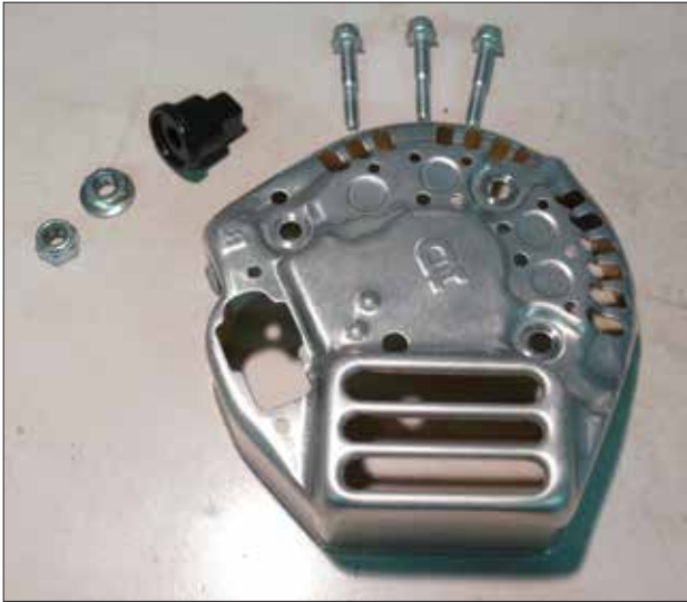
Remove the terminal shroud (left) to expose the brush holder and internal regulator.
