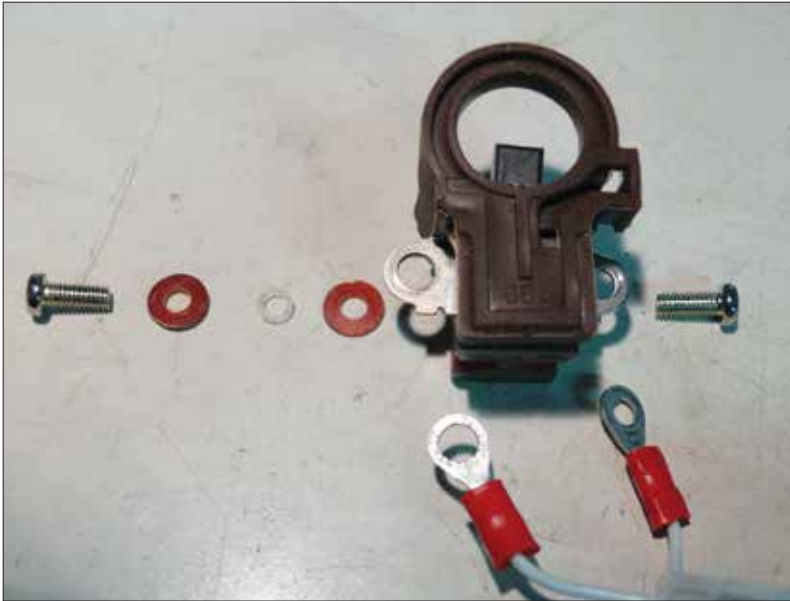
(Left) Brush holder and new components: two M4x10-mm screws, two fiber washers with 4-mm holes, one small piece of nylon tube (OD 5 mm, ID 4 mm, 1.5 mm long), and two terminated 18-gauge wires. (Right) The regulator is replaced by a mounting block with three holes: two for the original mounting screws and one with a captive nut that aligns with the hole in the regulator pointed to by the pen. This becomes the right-hand mounting point for the brush holder.
