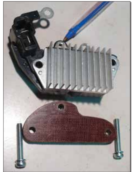
(Left) Brush holder and new components: two M4x10-mm screws, two fiber washers with 4-mm holes, one small piece of nylon tube (OD 5 mm, ID 4 mm, 1.5 mm long), and two terminated 18-gauge wires. (Right) The regulator is replaced by a mounting block with three holes: two for the original mounting screws and one with a captive nut that aligns with the hole in the regulator pointed to by the pen. This becomes the right-hand mounting point for the brush holder.
