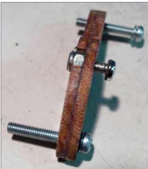
(Left) The mounting block is 1/4-inch thick and replaces the regulator after being cut to shape. It's made from two 1/8-inch thick pieces of canvas Bakelite, epoxied together and holding the nut. (Right) The mounting block attached to the alternator. Put one fiber washer where the left-hand brush-holder terminal was attached.
