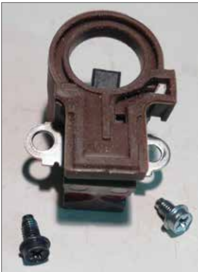
(Left) The brush holder is held in place with two screws. (Right) The alternator after removing the brush holder.
