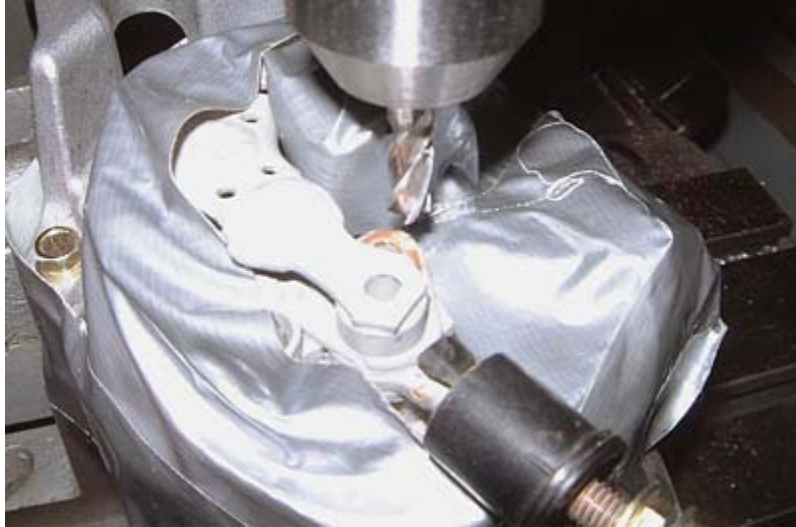
Although this image shows how Lynn used a mill to machine away the copper attachment, a handheld Dremel works fine, too.
