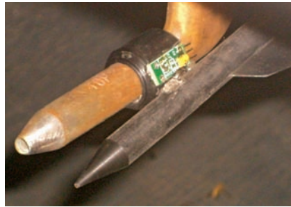
AOA Vane mounted next to Pitot tube.
