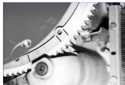
Typical timing marks on a Lycoming engine are located on the forward face of the ring gear. Note reference hole drilled in the starter housing (arrow).
