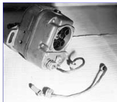
Timing adaptors for P-leads for Bendix S-20 magnetos can be fabricated from old parts or purchased outright. Note two different sizes of end connectors for different mag types.
